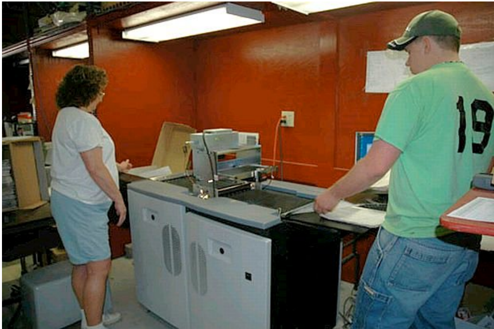
Dried documents are passed through high-speed scanners to be reprinted on clean paper
