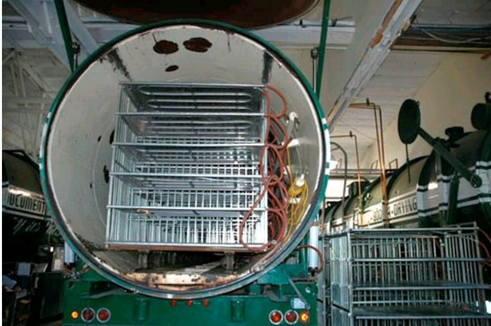
Inside a portable vacuum drying chamber at Document Reprocessors
